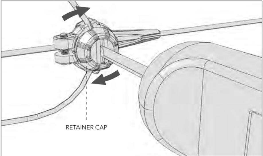
Re-position the HS1, then screw the retainer cap back into place
