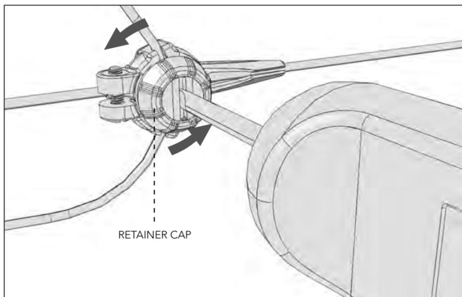
Loosening the retainer cap with provided RØDE screwdriver
