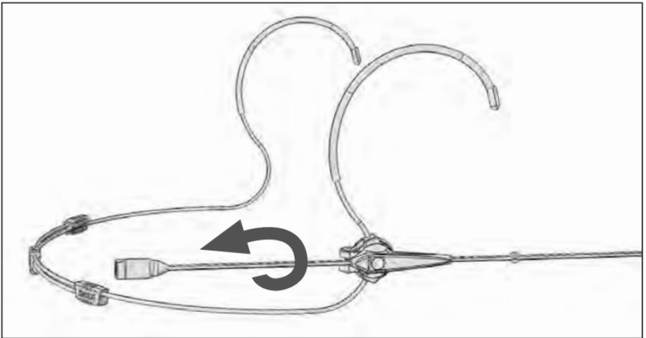
Push or pull the body of the HS1 through the retainer clasp using a twisting motion
