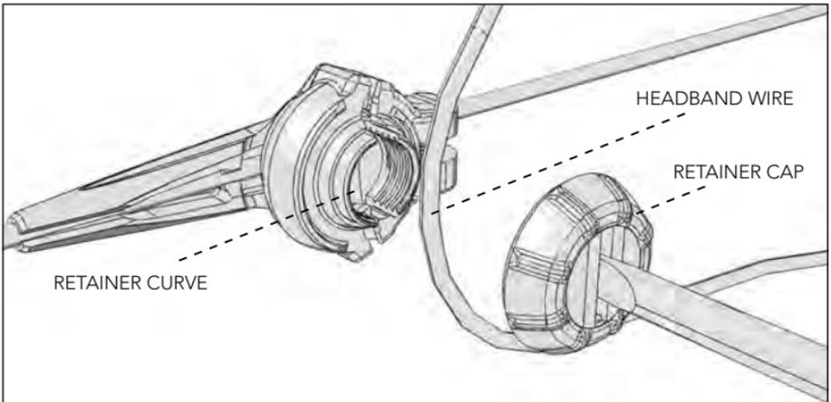
Completely unscrew the retainer cap
